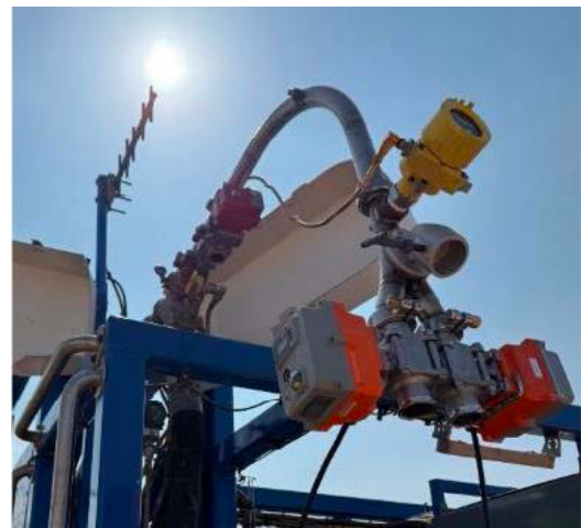
Figure 1: The powder splitter is a permanent attachment to the DriFlow system, creating dual-path powder delivery enabled by critical feeder system redundancies.
